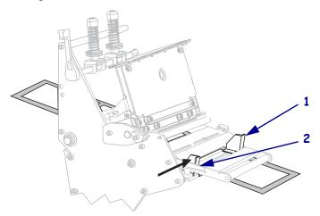
**16.** Tighten the thumb screw (not visible from this angle) that is located on the bottom of the outer media guide (**1**).
